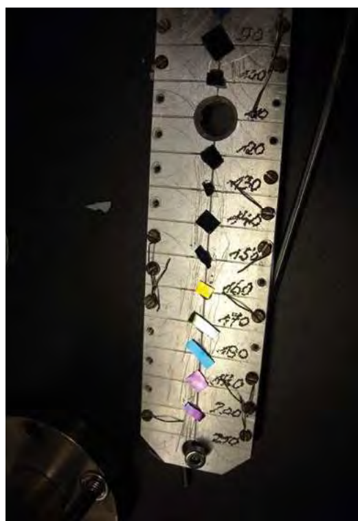
Figure 3: Thin films deposited on Si substrates can be investigated using RBS and NRA.
